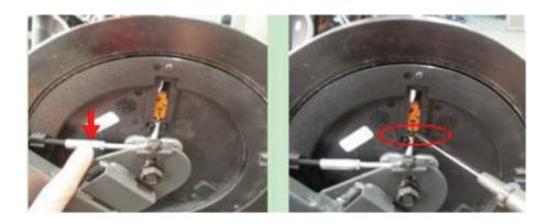
4. If all above conditions are ok, and the resistance is still too heavy, the magnet inside the ECB is defective. Replace the ECB.
